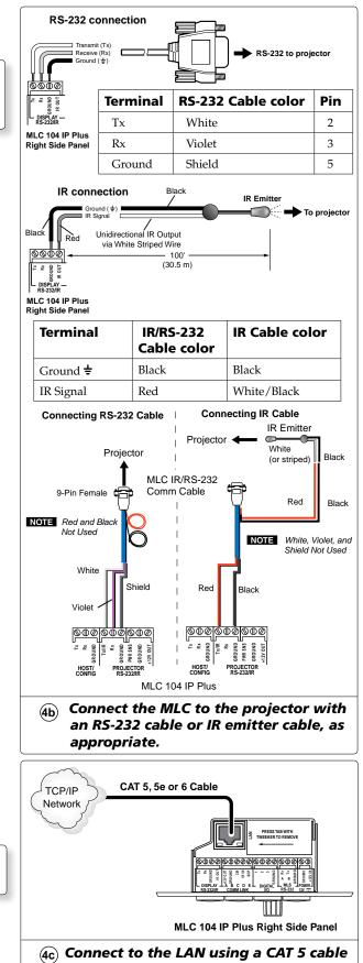
**c.** To use the MLC 104 IP Plus's IP Link feature, connect a network connected CAT 5, 5e, or 6 straight through cable to the MLC's RJ-45 LAN jack.
