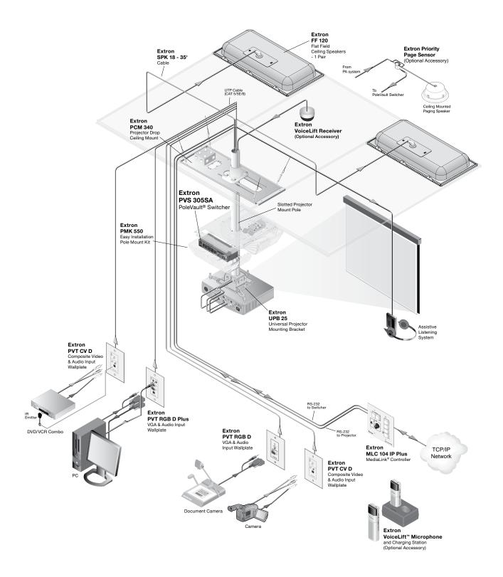
PoleVault System installation and wiring overview
