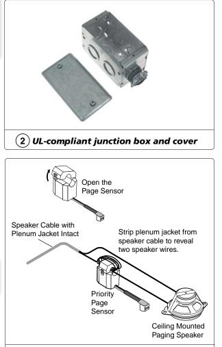
**4** Open the sensor and loop a wire around the sensor
