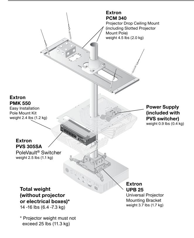
Ceiling mount installation diagram (with item weights) for PoleVault System
