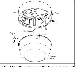
7) Align the arrows on the housing rim and the dome tab.
