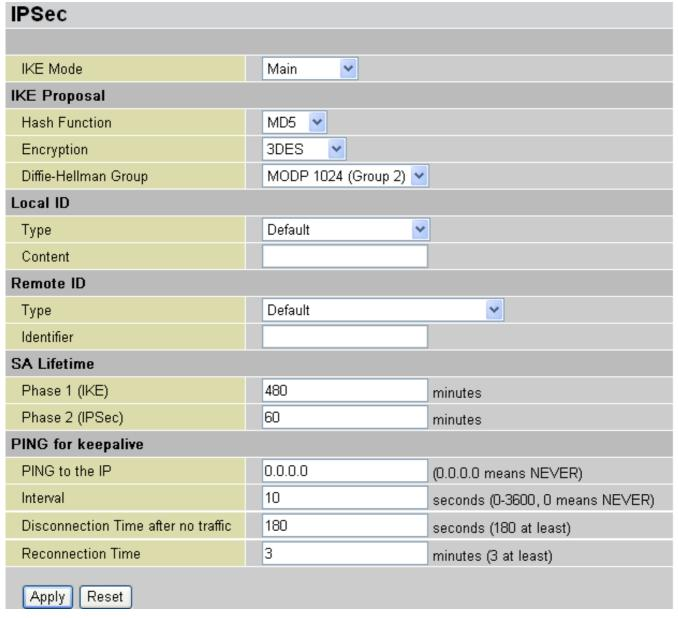
**IKE (Internet key Exchange) Mode:** Select IKE mode to Main mode or Aggressive mode. This IKE provides secured key generation and key management.
