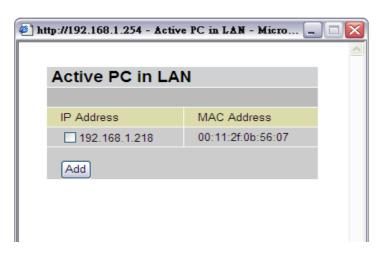
Active PC in LAN displays a list of individual Ethernet device's IP Address & MAC Address which connecting to the router.
