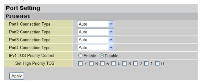
**Port # Connection Type:** Six options to choose from: Auto, 10M half-duplex, 10M full-duplex, 100M half-duplex, 100M full-duplex and Disable. Sometimes, there are Ethernet compatibility problems with legacy Ethernet devices, and you can configure different types to solve compatibility issues. The default is **Auto**, which users should keep unless there are specific problems with PCs not being able to access your LAN.
