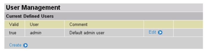
In order to prevent unauthorized access to your router's configuration interface, it requires all users to login with a password. You can set up multiple user accounts, each with their own password.
