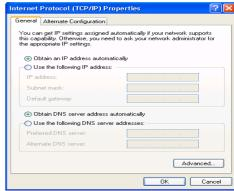
Figure 3.4: IP Address & DNS Configuration
