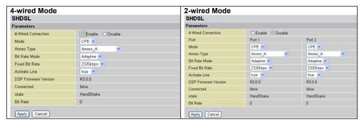
**4-Wired Connection:** BiPAC 8520 supports either 2-wire and 4-wires SHDSL connection. Activate the device to 4-wired by enabling the function; otherwise, disable it to be used as 2-wire mode connection.
