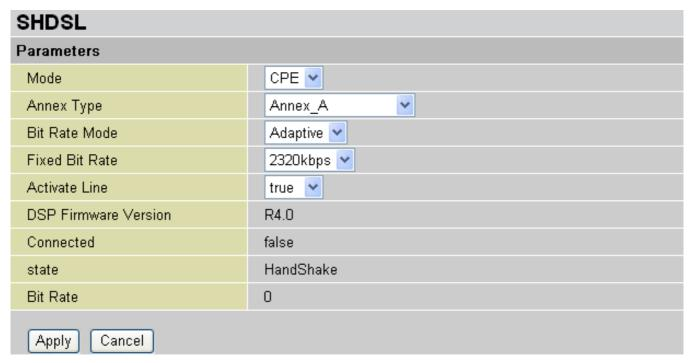
**Mode**: The SHDSL device can function as a CPE (Customer Premises Equipment) or CO. Select CPE mode when the BiPAC 8501 is connecting to your ISP.
