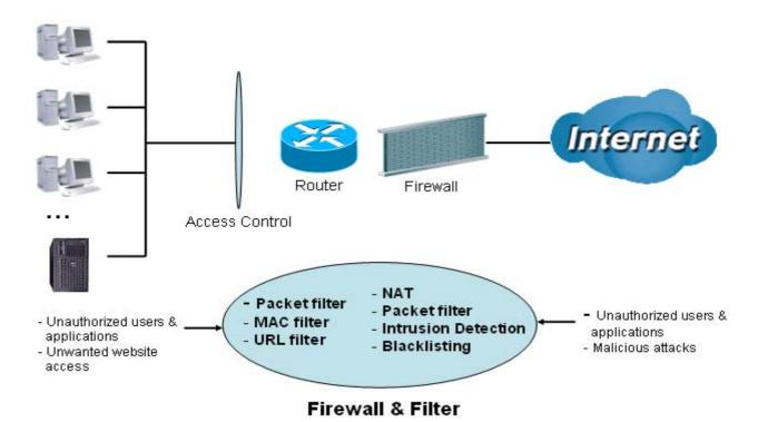
**Firewall**: Prevents access from outside your network. The router provides three levels of security support:
